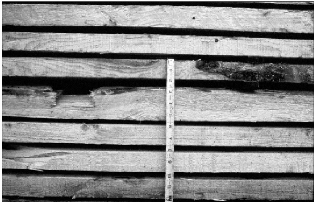
Figure 5.—Excessive between-board variation.
